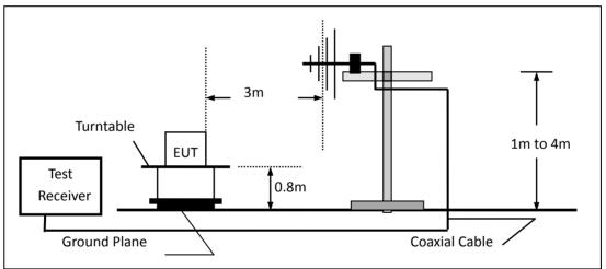
(c) For radiated emissions above 1000MHz
