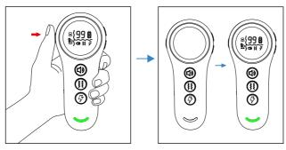
Turn on the Receiver/Bark Control Collar by pressing and holding the Power Button for 3 seconds with vibration, as the white LED Indicator light blinks regularly.
