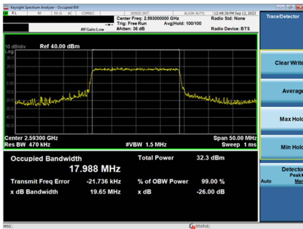
Plot 7-45. Occupied Bandwidth Plot (LTE Band 41(PC3) - 20MHz QPSK - Full RB - Ant2)
