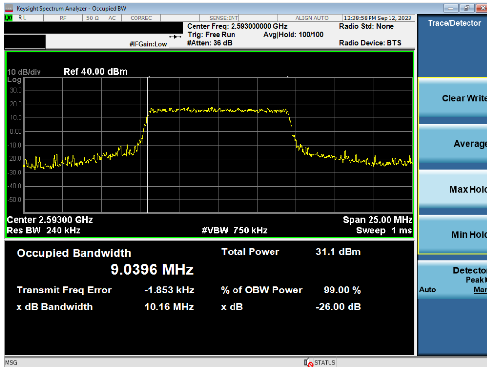
Plot 7-6. Occupied Bandwidth Plot (LTE Band 41(PC3) - 10MHz 16-QAM - Full RB - Ant1)
