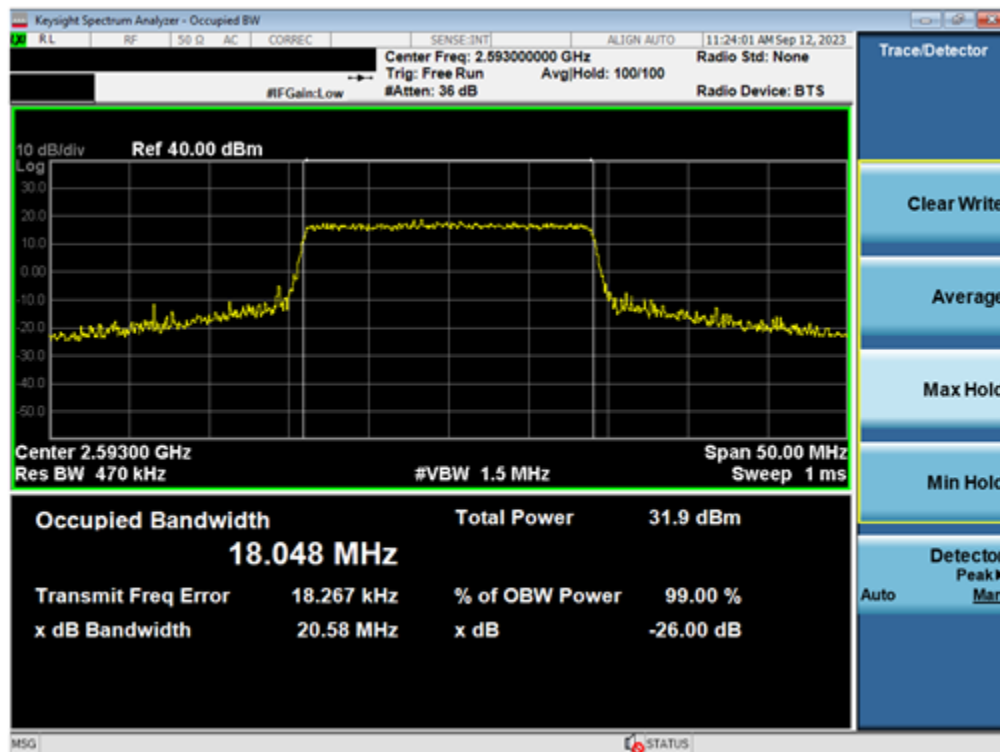
Plot 7-2. Occupied Bandwidth Plot (LTE Band 41(PC3) - 20MHz 16-QAM - Full RB - Ant1)
