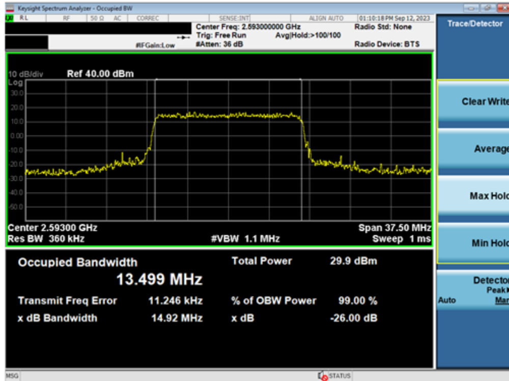
Plot 7-47. Occupied Bandwidth Plot (LTE Band 41(PC3) - 15MHz QPSK - Full RB - Ant2)
