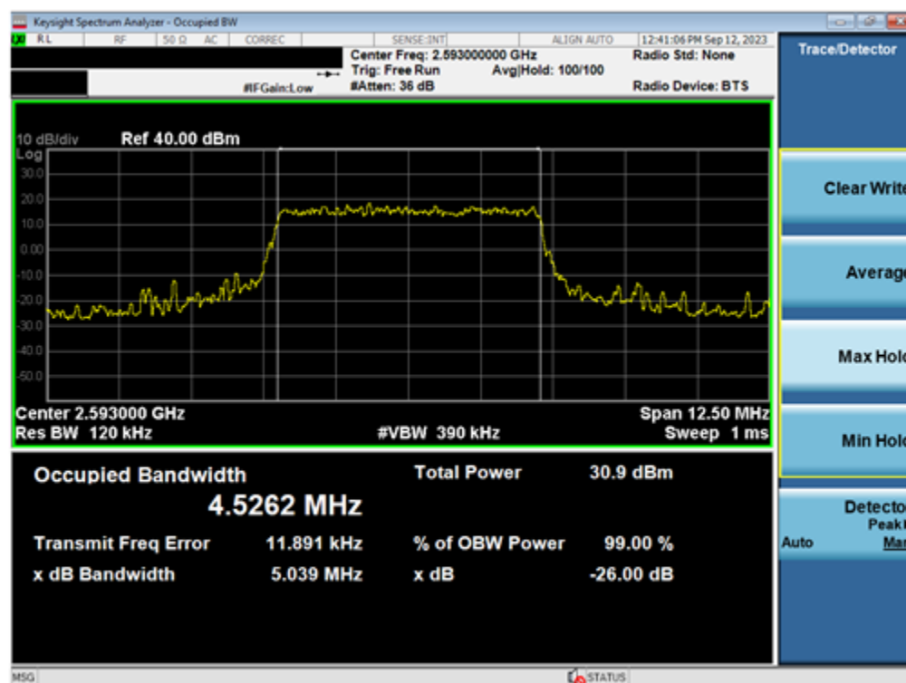
Plot 7-8. Occupied Bandwidth Plot (LTE Band 41(PC3) - 5MHz 16-QAM - Full RB - Ant1)
