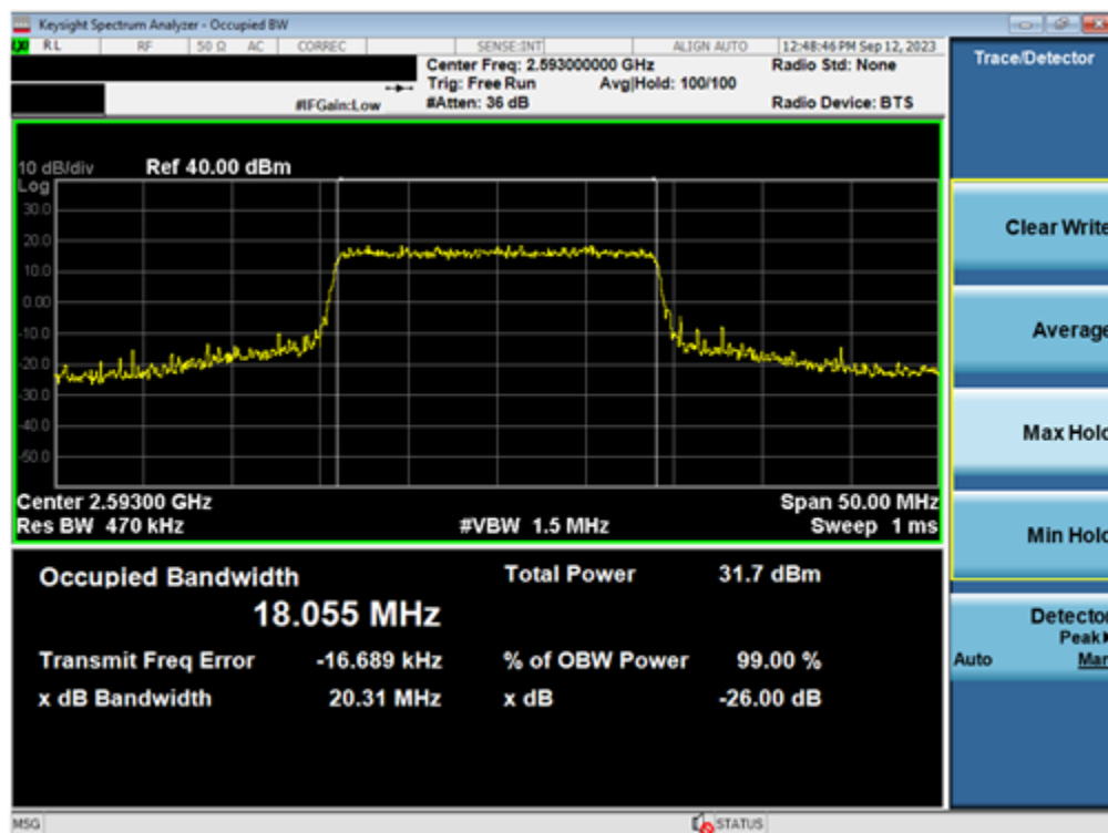
Plot 7-46. Occupied Bandwidth Plot (LTE Band 41(PC3) - 20MHz 16-QAM - Full RB - Ant2)
