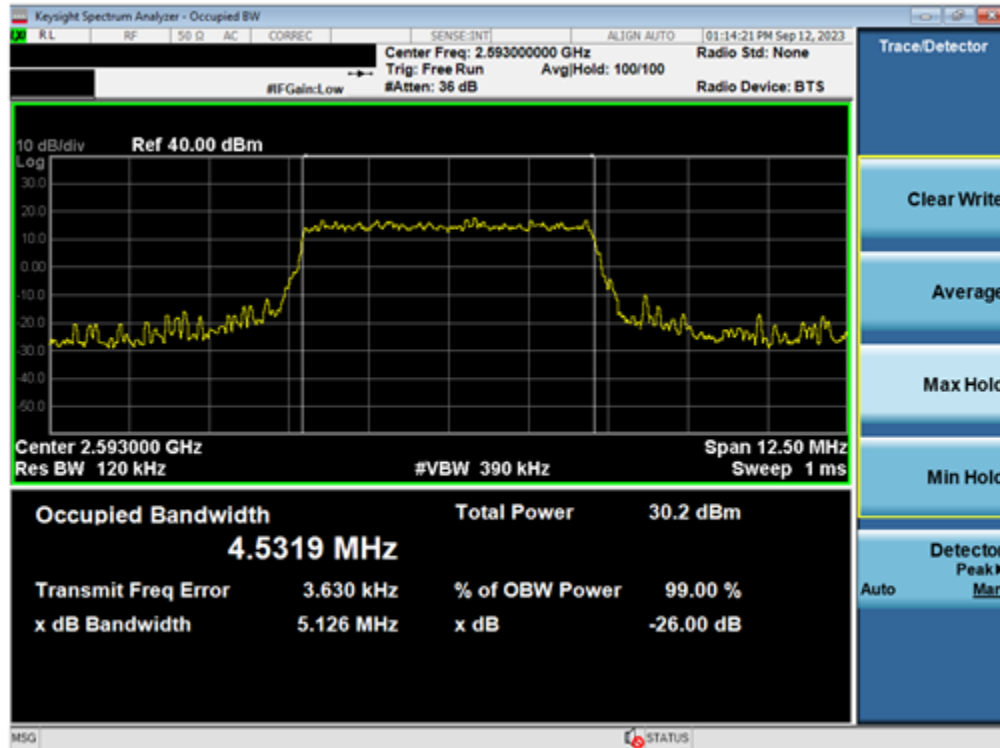
Plot 7-51. Occupied Bandwidth Plot (LTE Band 41(PC3) - 5MHz QPSK - Full RB - Ant2)
