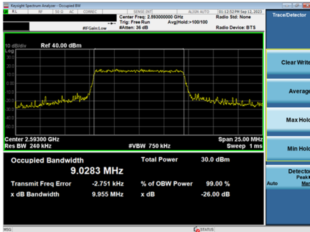
Plot 7-50. Occupied Bandwidth Plot (LTE Band 41(PC3) - 10MHz 16-QAM - Full RB - Ant2)
