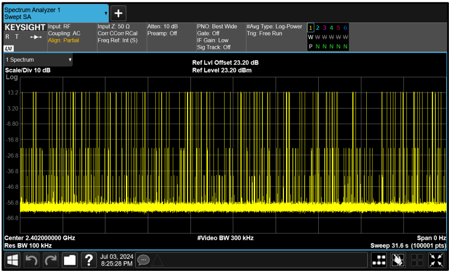
Figure 49 - GFSK - 2402 MHz Accumulated Transmit Time
