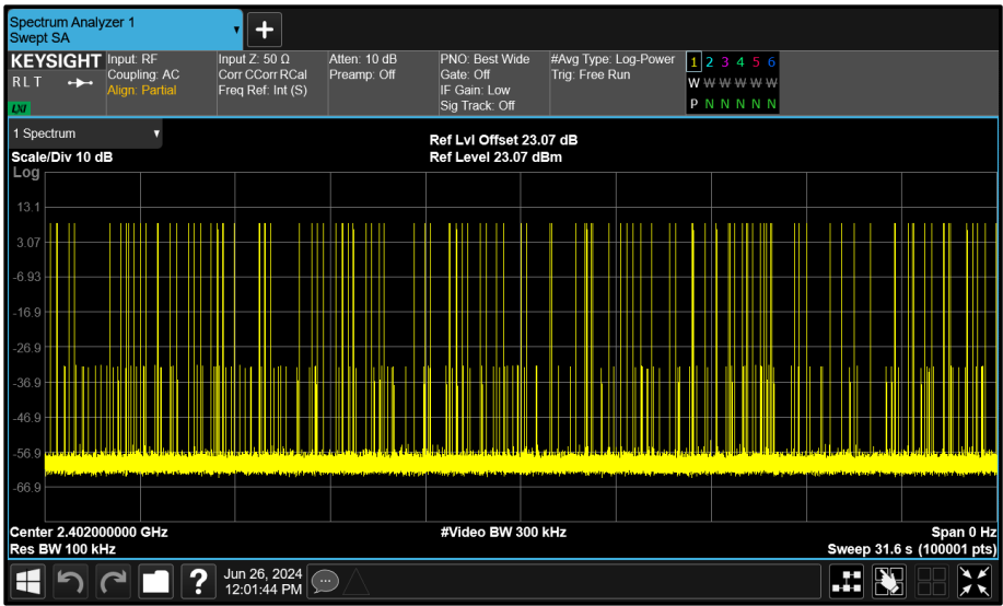
Figure 53 - \pi/4 DQPSK - 2402 MHz Accumulated Transmit Time
