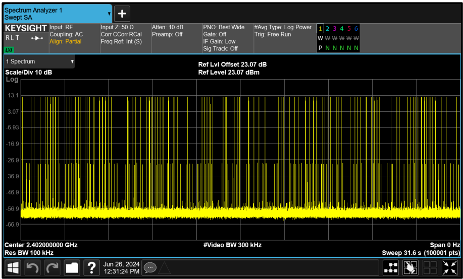
Figure 57 - 8-DPSK - 2402 MHz Accumulated Transmit Time
