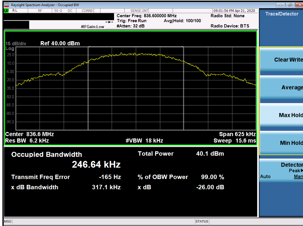
Plot 7-1. Occupied Bandwidth Plot (Cellular GPRS Mode)
