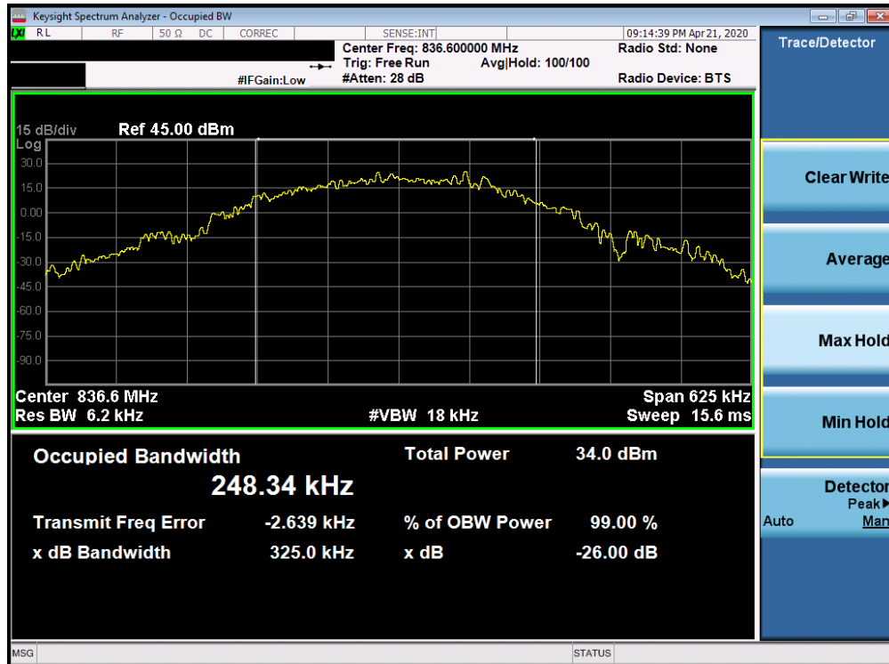
Plot 7-2. Occupied Bandwidth Plot (EDGE850 Mode)
