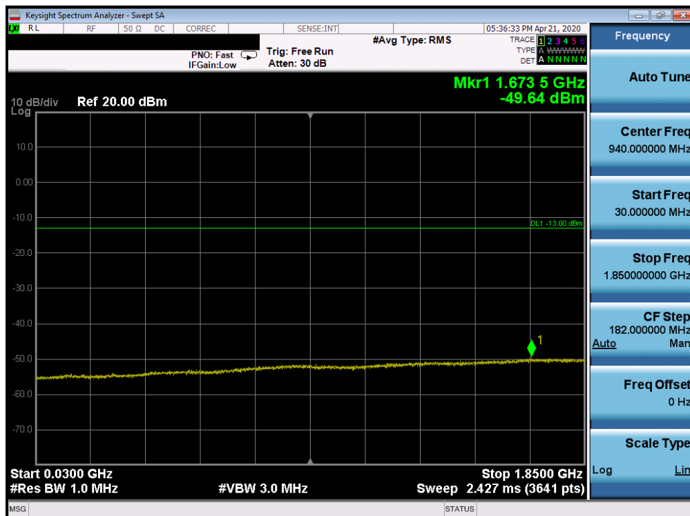
Plot 7-40. Conducted Spurious Plot (PCS CDMA Mode - Mid Channel)
