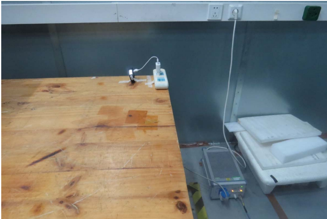
Picture 2 Conducted Emission Test Setup
