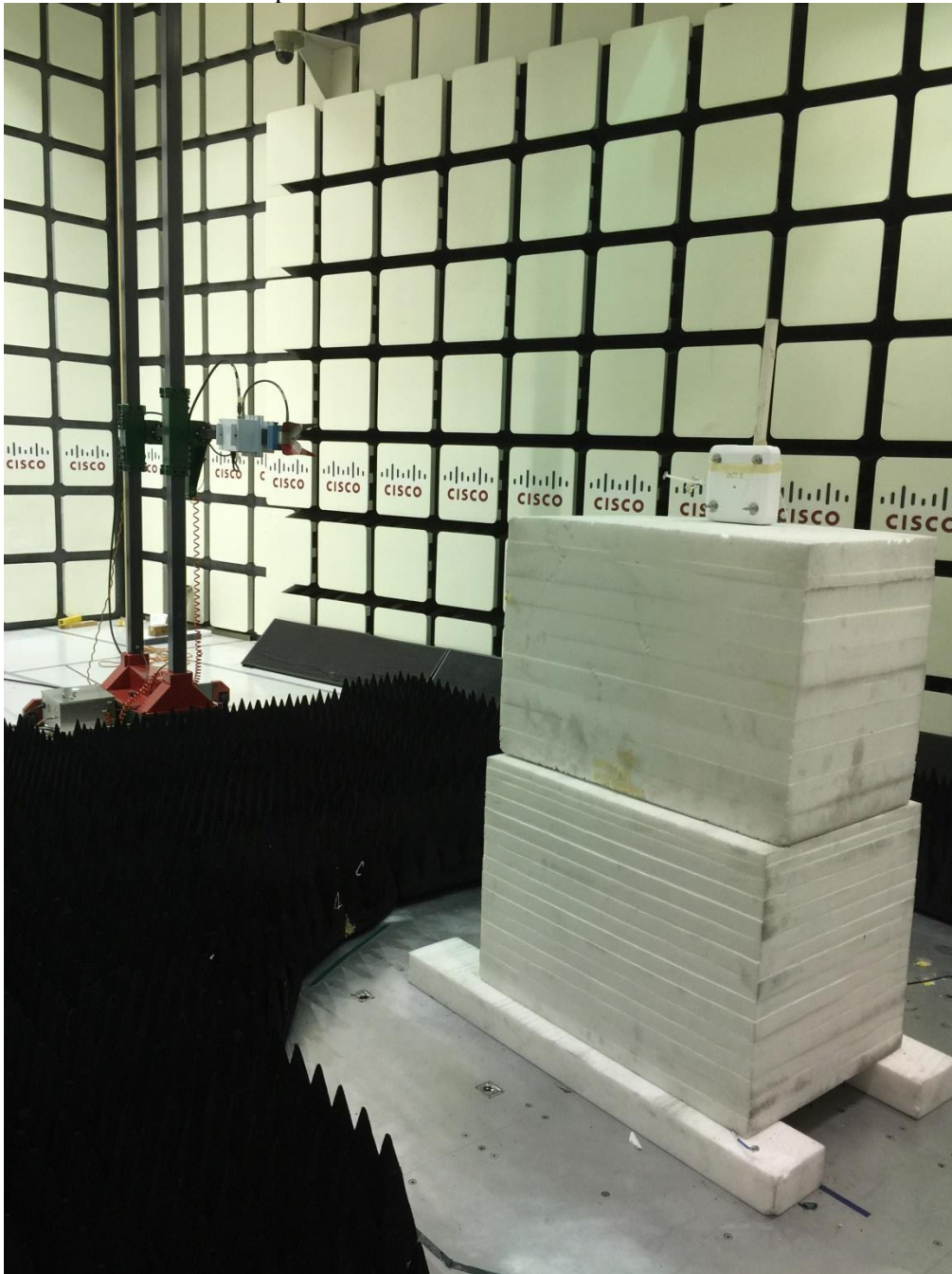
Radiated Emissions setup above 1GHz
