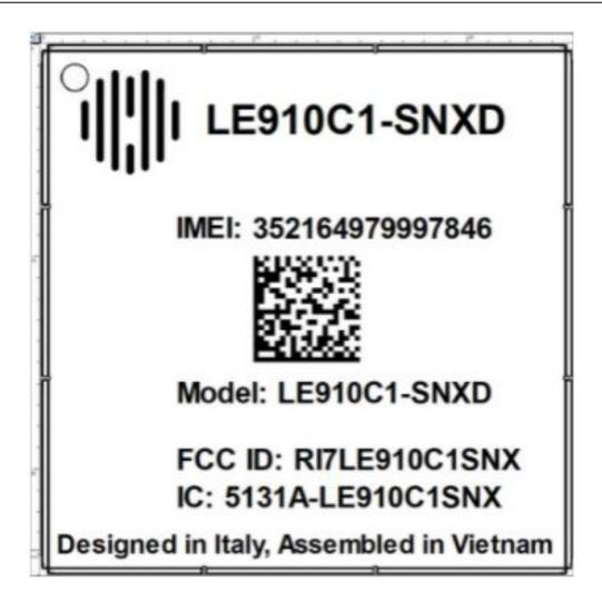
The label is laser engraved on the metallic shield of the module. The above is just the appearance of the information included in the engraving.
