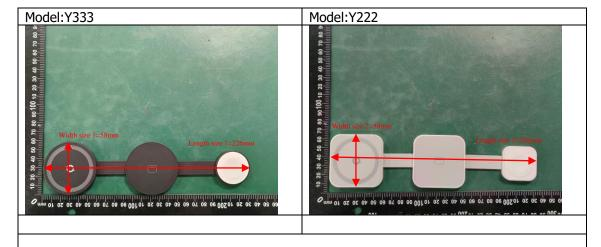
For model Y333 and Y222, the product enclosure shape is not the same, Y333 is round and model Y222 is square. But model Y333 and Y222 have have the same length and width. Size: length(226mm)\*width(58mm)
