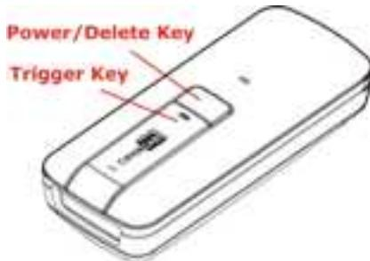
Note: (1) To turn off the scanner, press the [Power/Delete] key for 2 seconds. The scanner will respond with two short beeps (high tone) and the LED will become solid red. Release the key. Otherwise, let the scanner turn off automatically in specific circumstances. Refer to settings of "[Auto Power Off](#)".
