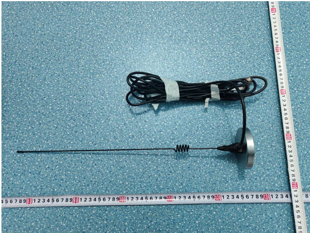
Radio Antenna (902-928MHz, only RX)
