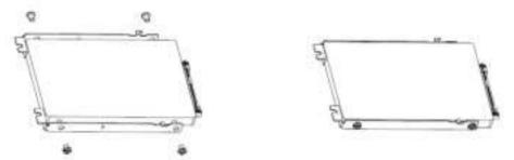
a. The disk is facing up, with the R bracket at the bottom and the L Bracket at the top.
