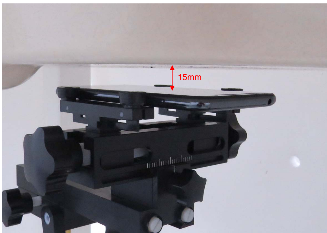
Picture 6: Front Side, the distance from handset to the bottom of the Phantom is 15mm (ATU-L11)
