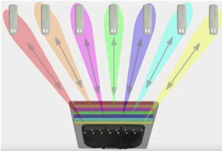
Figure 55 PMP 450m Series AP antenna beam
