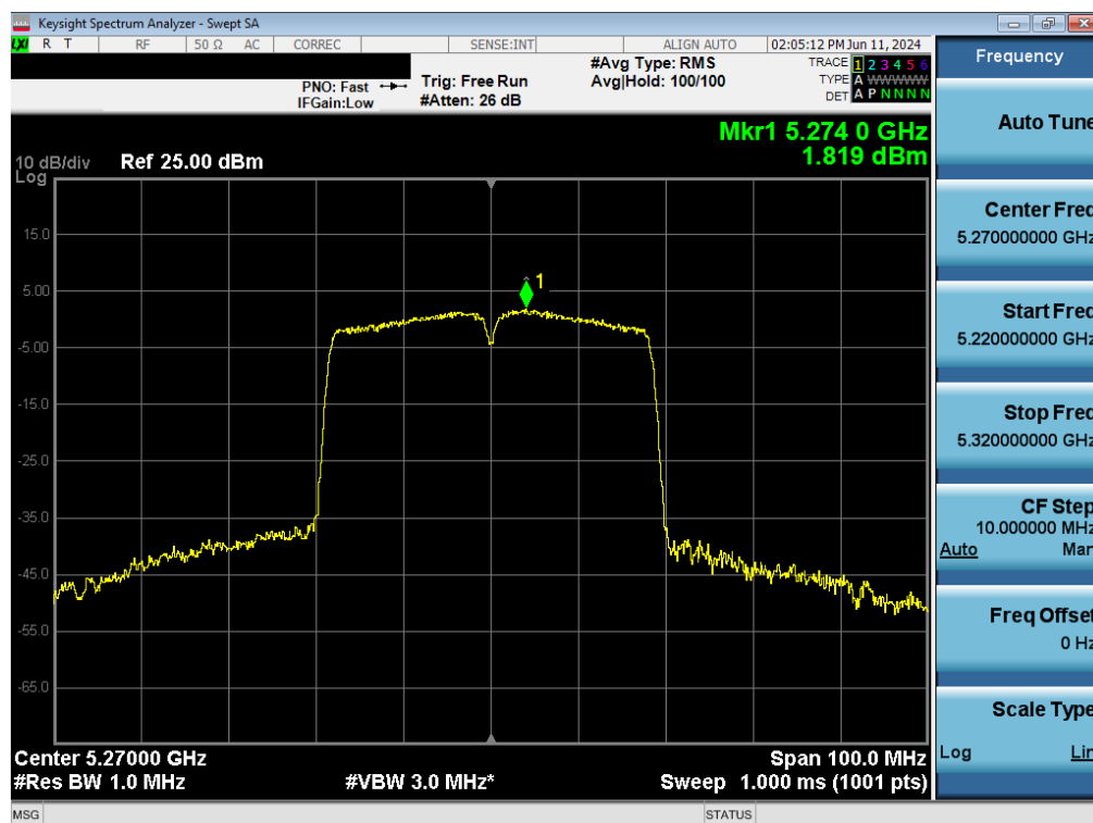
Plot 7-95. Power Spectral Density Plot MIMO ANT1 (40MHz BW 802.11n (UNII Band 2A) – Ch. 54)
