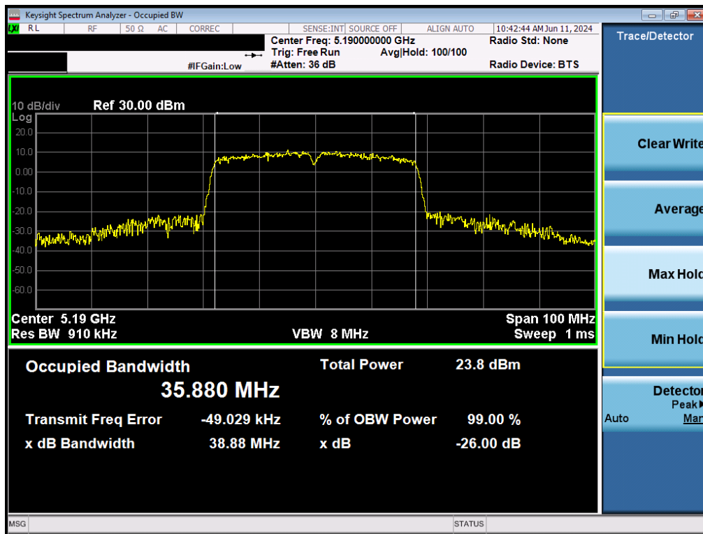
Plot 7-29. 26dB Bandwidth Plot MIMO ANT2 (40MHz BW 802.11n (UNII Band 1) – Ch. 38)
