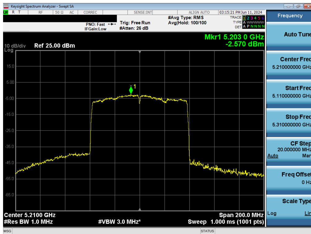
Plot 7-88. Power Spectral Density Plot MIMO ANT1 (80MHz BW 802.11ac (UNII Band 1) – Ch. 42)
