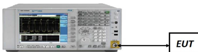
Figure 7-2. Test Instrument & Measurement Setup
