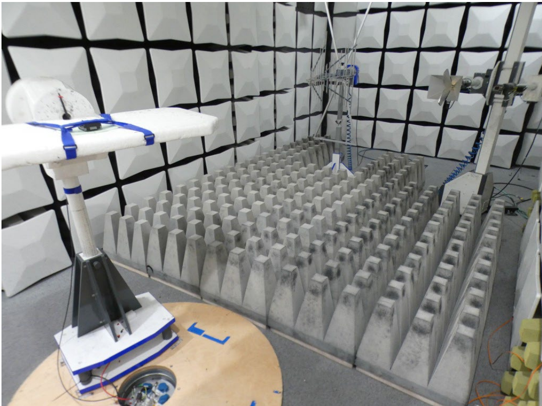
Photo 3: Setup Spurious Emissions Radiated (FAC), > 1GHz
