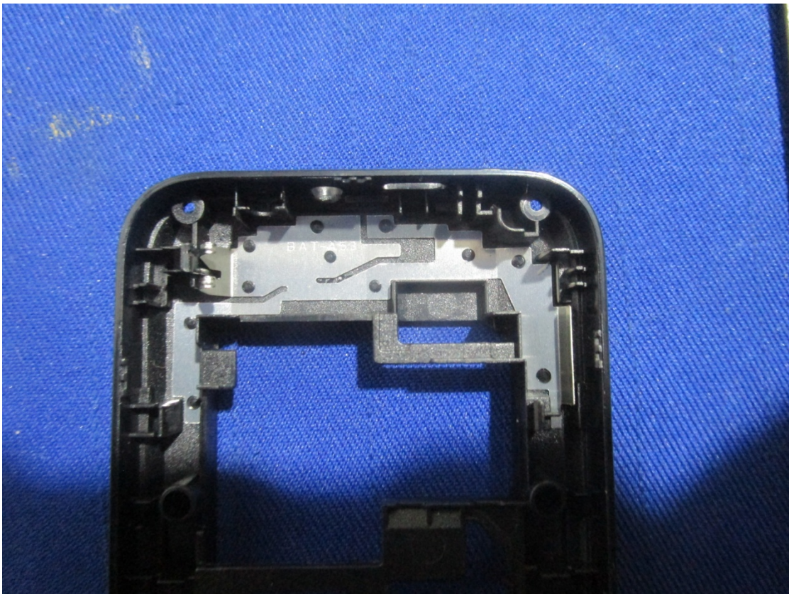
GSM Antenna View
