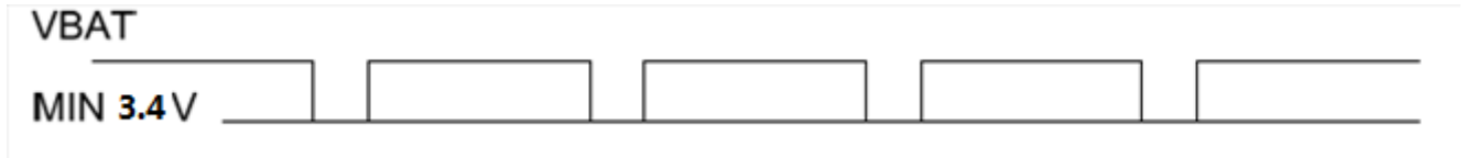
Figure 4.4: VBAT lowest voltage drop
