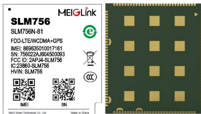
Figure 48: Module top and bottom views
