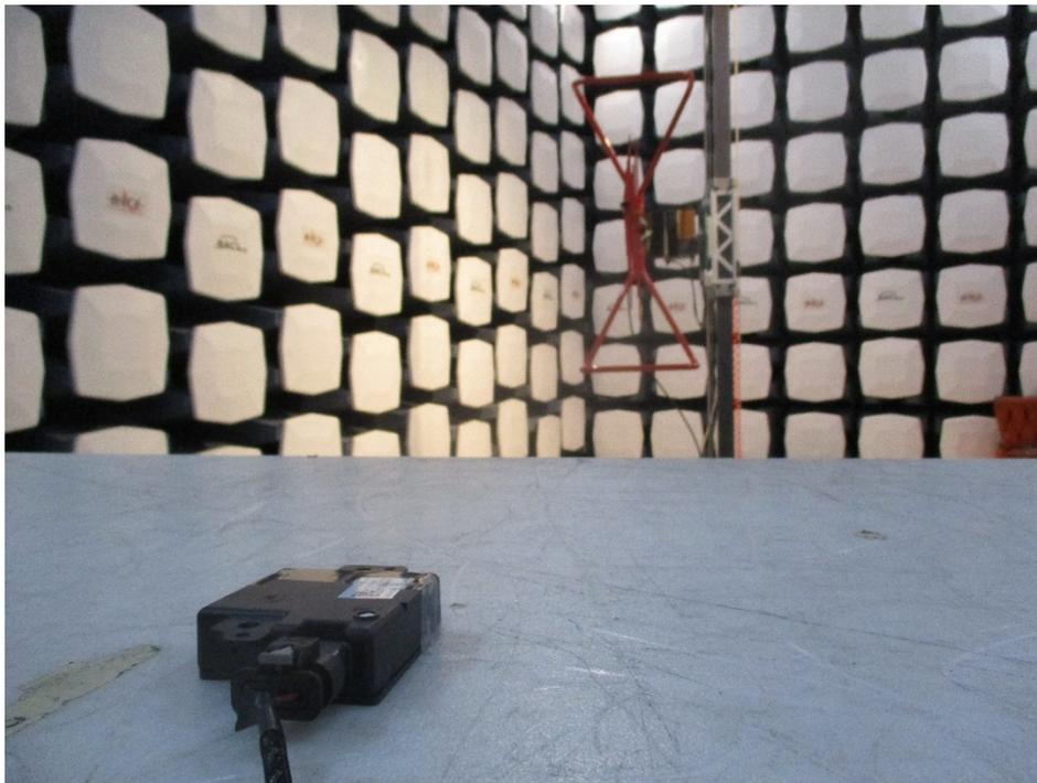
**1.5 Front View EUT Test Setup at 1 Meter (1-18GHz)**
