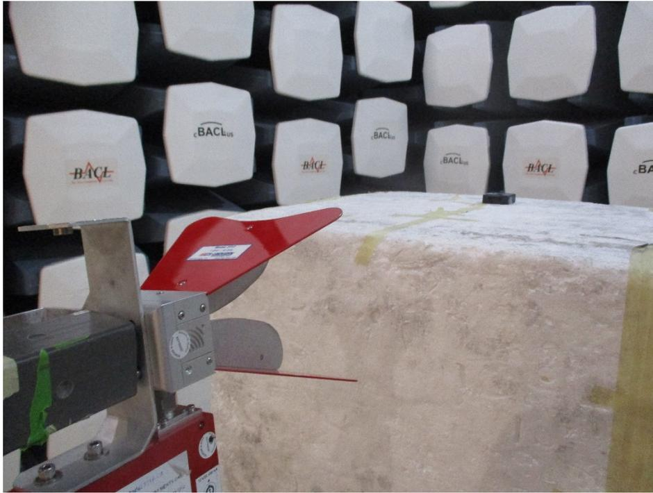
**1.6 Rear View EUT Test Setup at 1 Meter (1-18GHz)**
