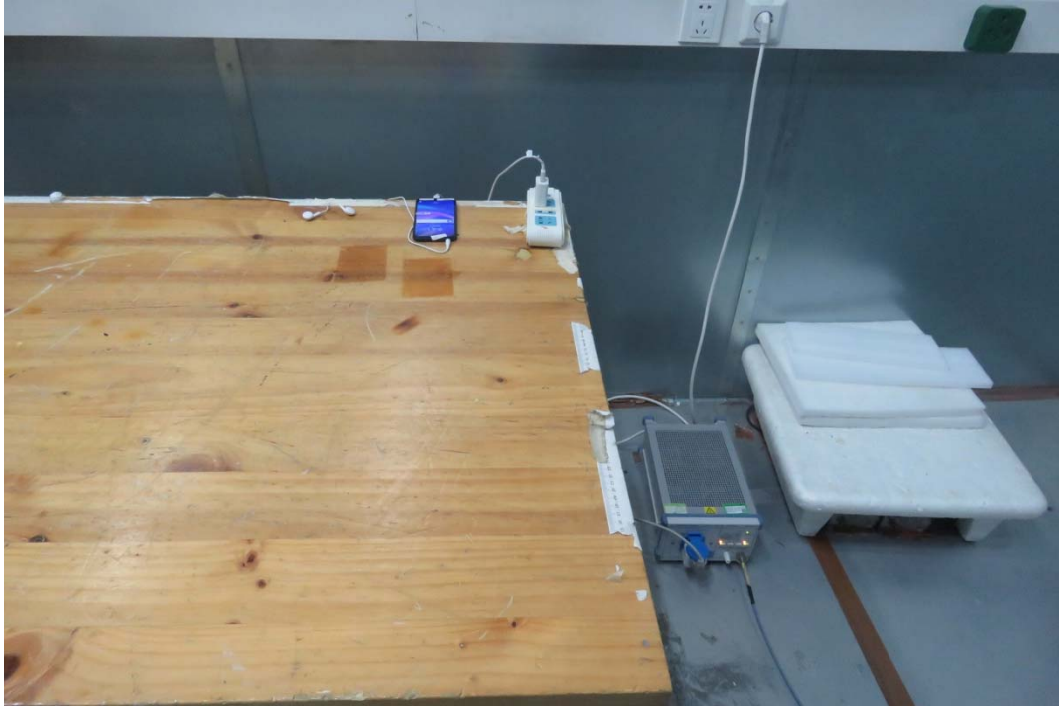
Picture 2 Conducted Emission Test Setup
