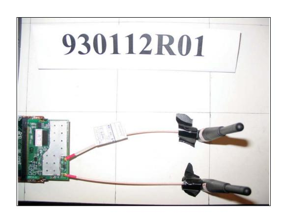
RADIATED EMISSION TEST (Test Mode: PIFA Antenna)
