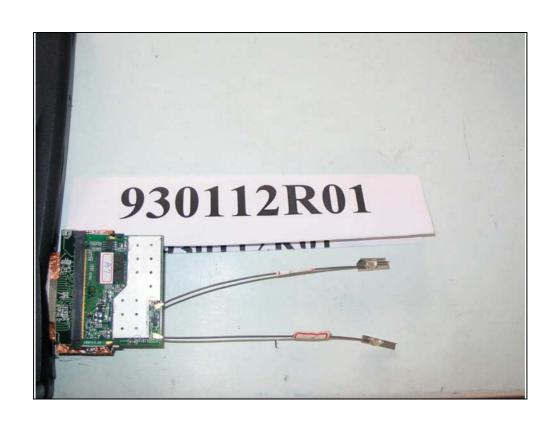
RADIATED EMISSION TEST (Test Mode: Dipole Antenna)
