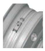
Place the sensor on bottom of wheel, ensuring arrow direction the same side of valve.
