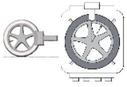
Break the tyre bead, ensuring the valve is on the opposite side of the wheel from the bead breaker blade. When the tyre is dismounted the valve must be located at 1 o'clock to the tyre fitting head.
