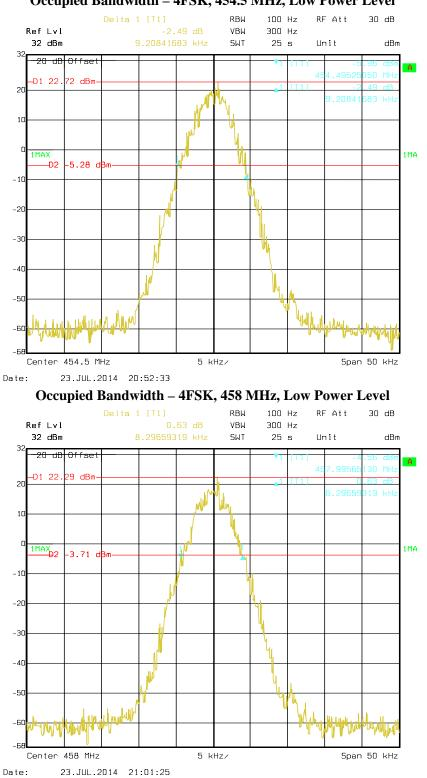
Occupied Bandwidth - 4FSK, 454.5 MHz, Low Power Level
