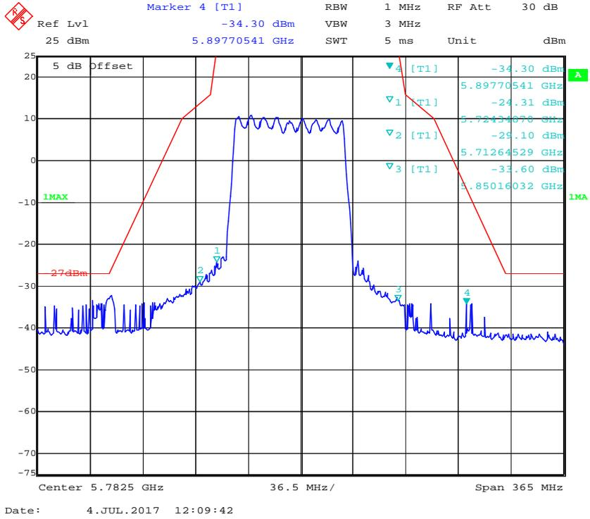
**MIMO Mode:**(the antenna gain was offset in the display, all emissions under limit 3dB, so combined results meet the requirement)
