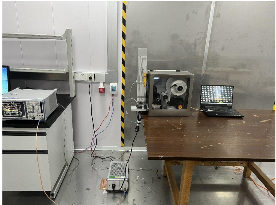
Conducted Emission Test Setup
