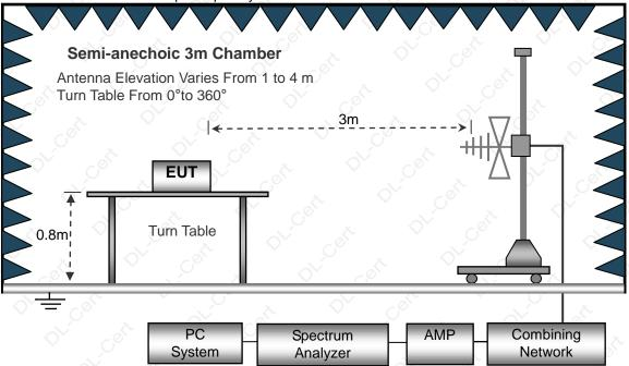
(C) Radiated Emission Test-Up Frequency Above 1GHz
