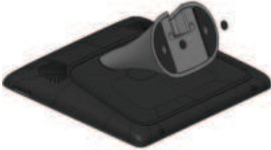
9 Install the threaded posts (all thread) into the base of the charging station.
