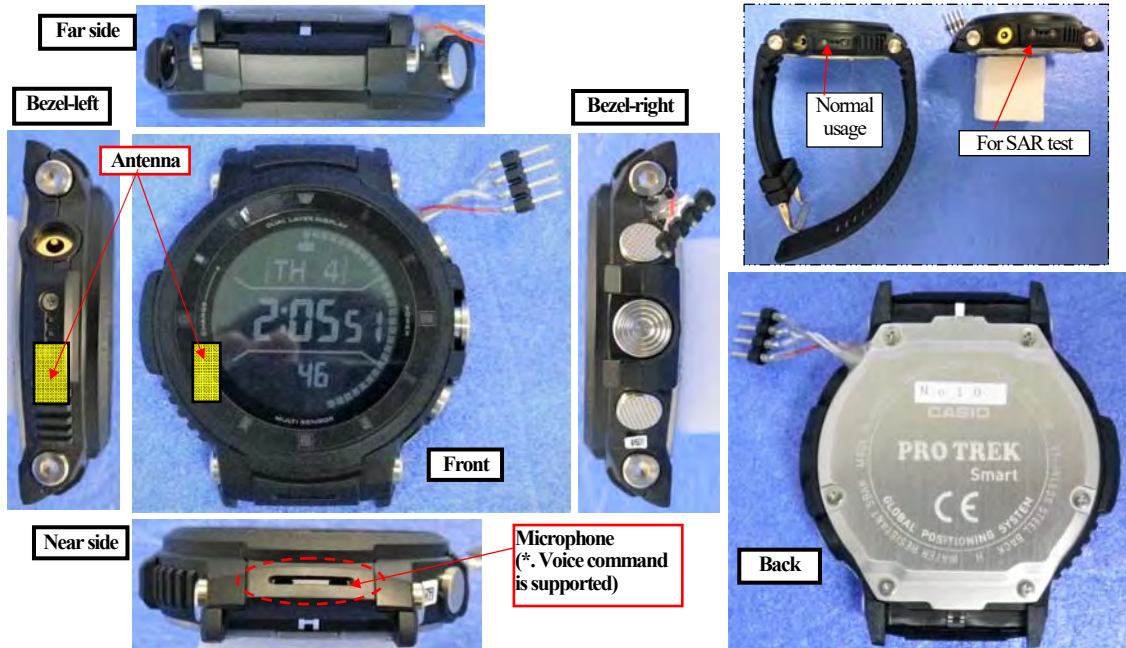
Antenna location and antenna distance [Unit: mm]
