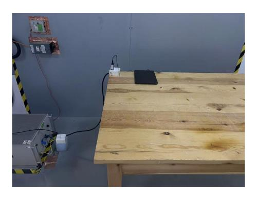
Set-up for Radiated Emission (RE), Below 1GHz
