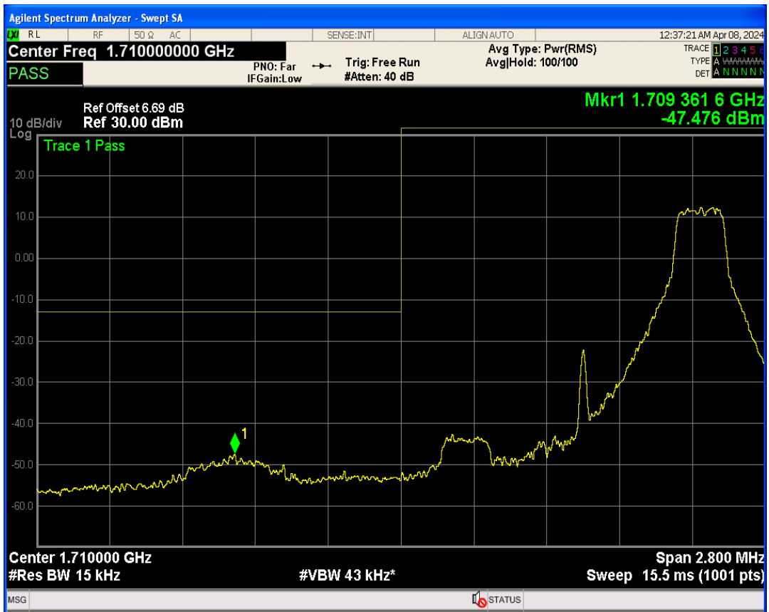
Band4 16QAM BW=1.4MHz Channel=19957 RB Size=6 Position=#0
