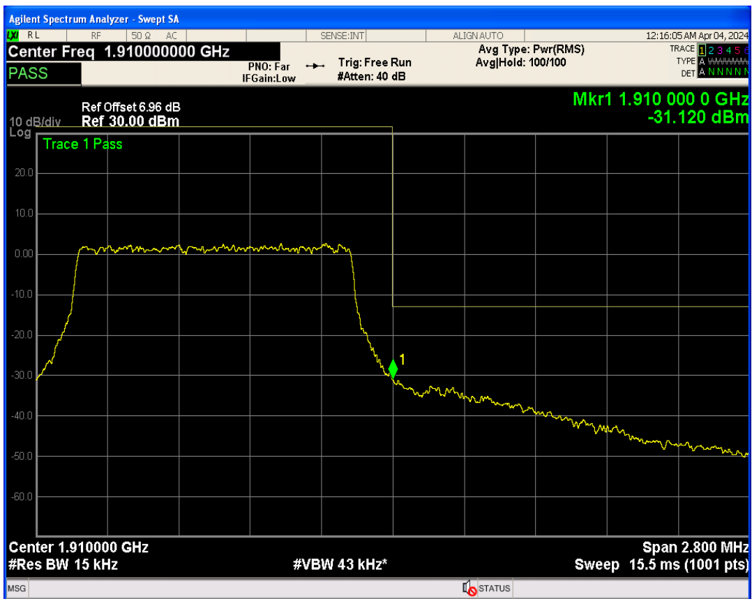
Band2 QPSK BW=3MHz Channel=18615 RB Size=1 Position=#0
