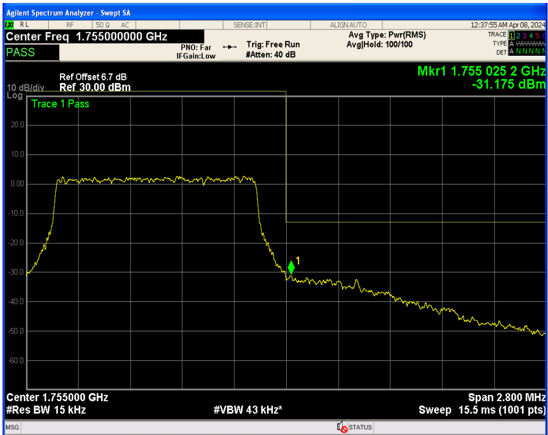
Band4 QPSK BW=3MHz Channel=19965 RB Size=1 Position=#0
