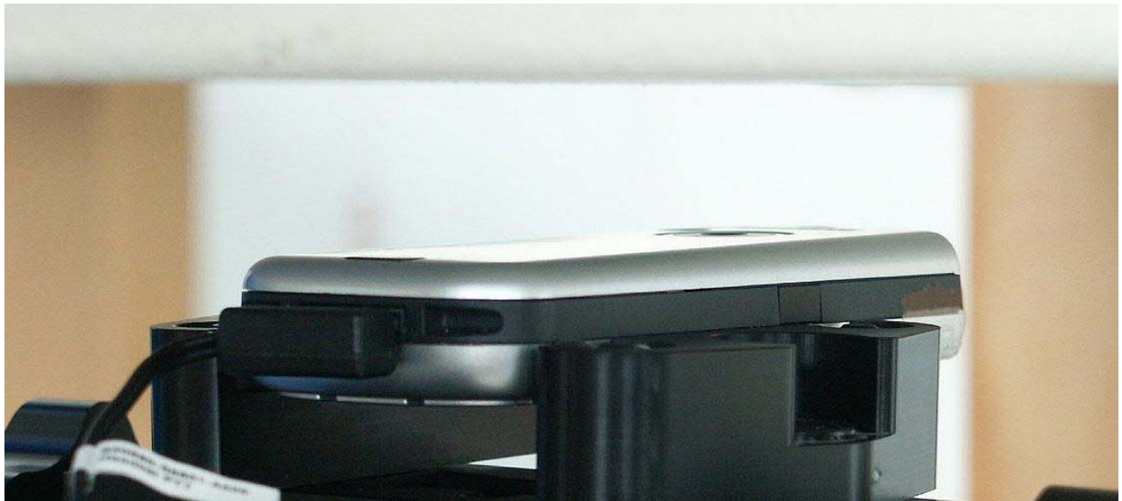
Fig. 31: Body worn configuration, GSM headset HHS-510, antenna towards the phantom (distance = 20 mm).
