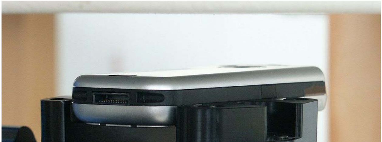
Fig. 30: Body worn configuration, GSM, antenna towards the phantom (distance = 20 mm).
