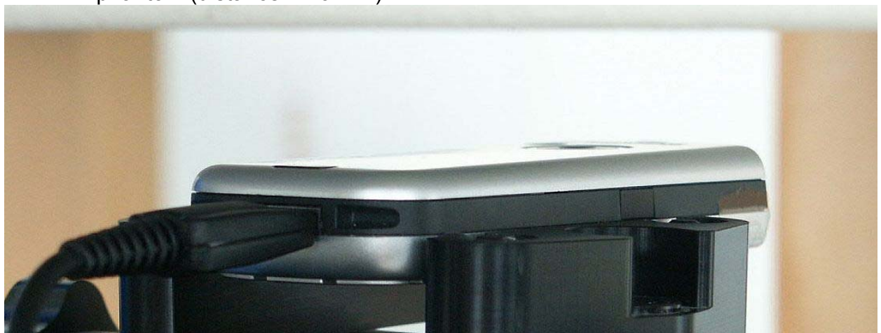
Fig. 32: Body worn configuration, GPRS (Class 10) with data cable DCA-500, antenna towards the phantom (distance = 20mm).
