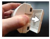
STEP REMOVE BATTERY TAB
