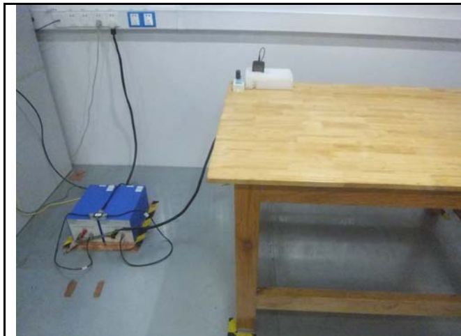
Conducted Emissions Test Setup Front View
