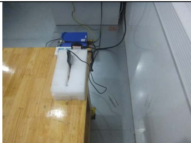
Conducted Emissions Test Setup Side View
