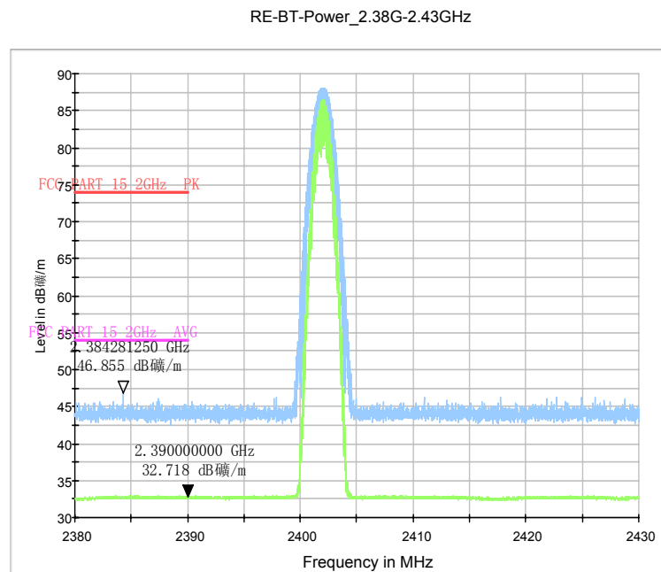
Fig.85. Radiated emission (Power): 8DPSK, low channel
