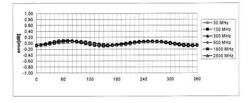
Axial Isotropy Error < ± 0.2 dB
