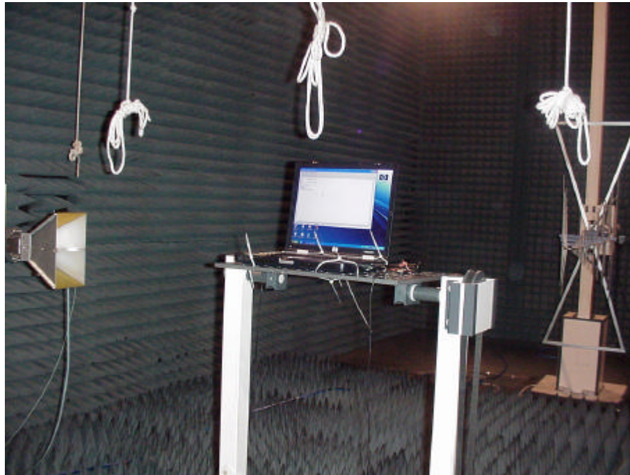
Picture 3 : Setup for radiated measurements (EUT in the Laptop)
