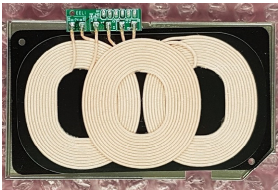
Charging coil element with connector, ferrite plate and metal shield, view from top and bottom side.
