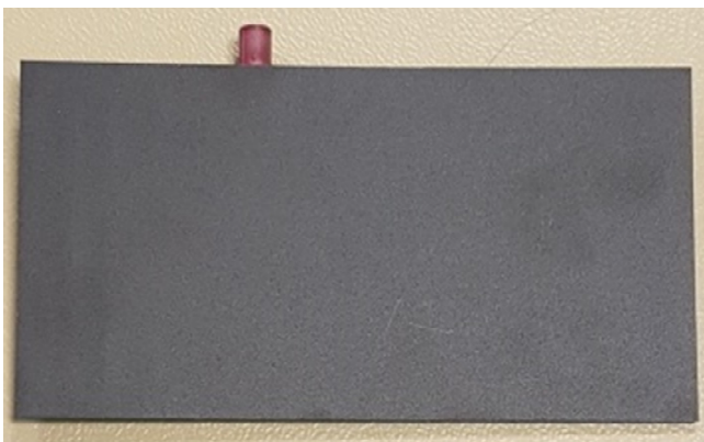
Antenna-PCB (NFC-Antenna and GSM-Coupling-Antenna), top and bottom view. The violet Fakra-Connector connects the GSM Roof-Antenna and the coupling Antenna (Red marked). The NFC-Antenna is yellow marked in the inner Layer of the PCB.
