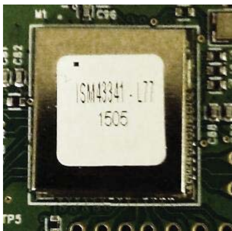
EUT Radio with shielding
