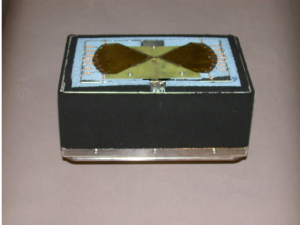
Tx antenna complete. Showing absorbents both inside shields and also on outside of outer shield.
