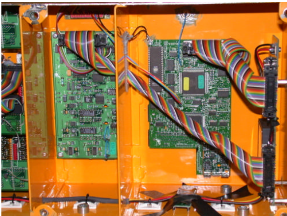
CPU board and timing circuitry
