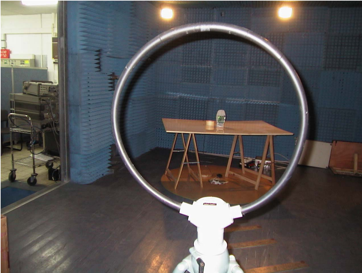
Radiated Emission Test Setup up to 30MHz
