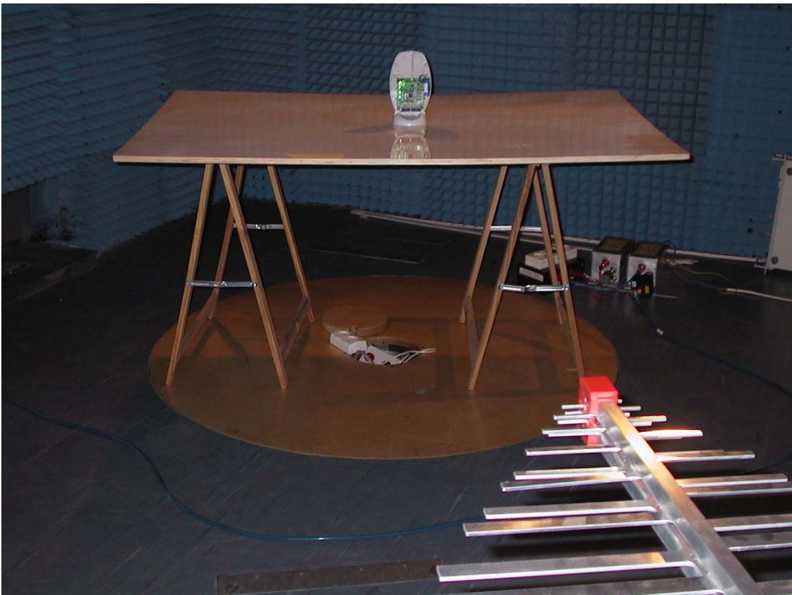
Radiated Emission Test Setup 30MHz-1GHz
