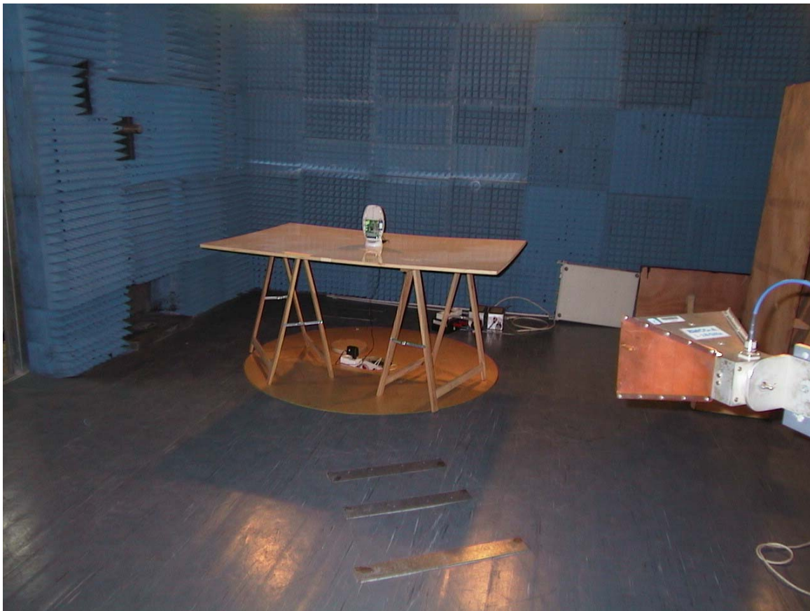
Radiated Emission Test Setup 1GHz-18GHz
