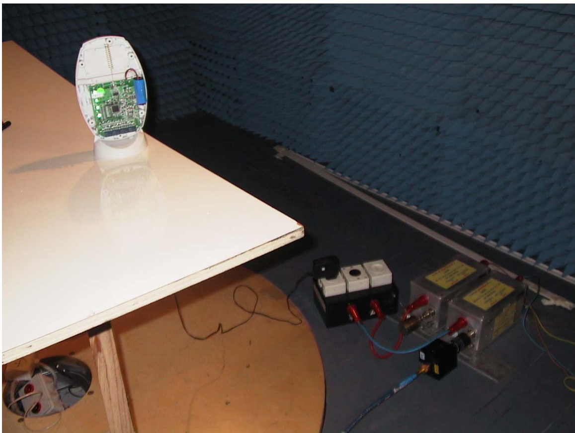
conducted Emission Set Up
