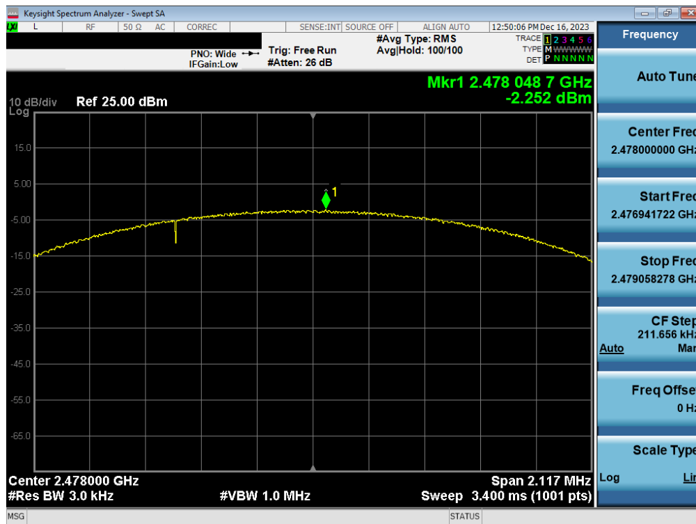
Plot 7-53. Power Spectral Density Plot Antenna WF7b (Bluetooth (LE), 2Mbps, ePA – Ch. 38)
