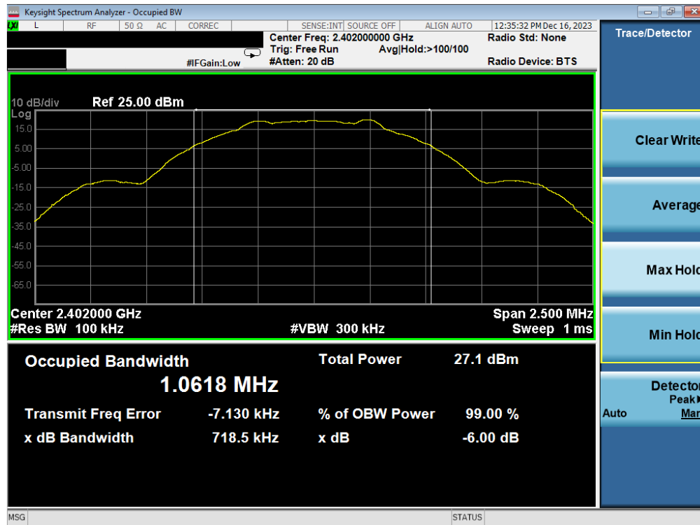
Plot 7-1. 6dB BW & 99% OBW Plot Antenna WF7b (Bluetooth (LE), 1Mbps, ePA – Ch. 0)
