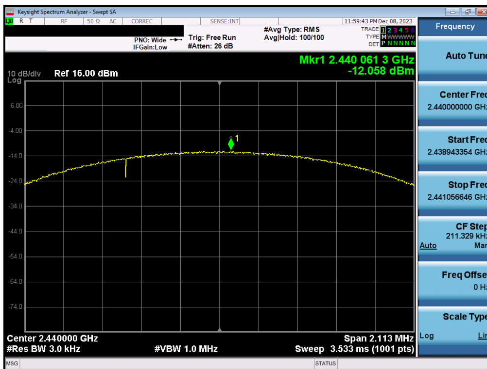
Plot 7-35. Power Spectral Density Plot Antenna WF2b (Bluetooth (LE), 2Mbps, iPA – Ch. 19)
