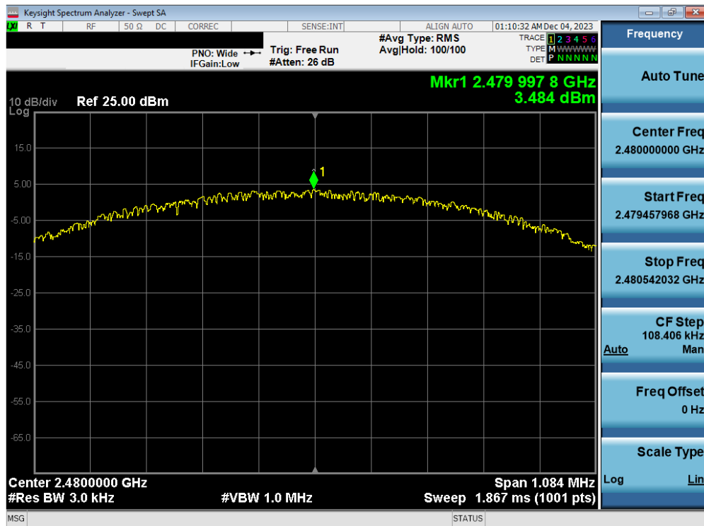
Plot 7-27. Power Spectral Density Plot Antenna WF2b (Bluetooth (LE), 1Mbps, ePA – Ch. 39)
