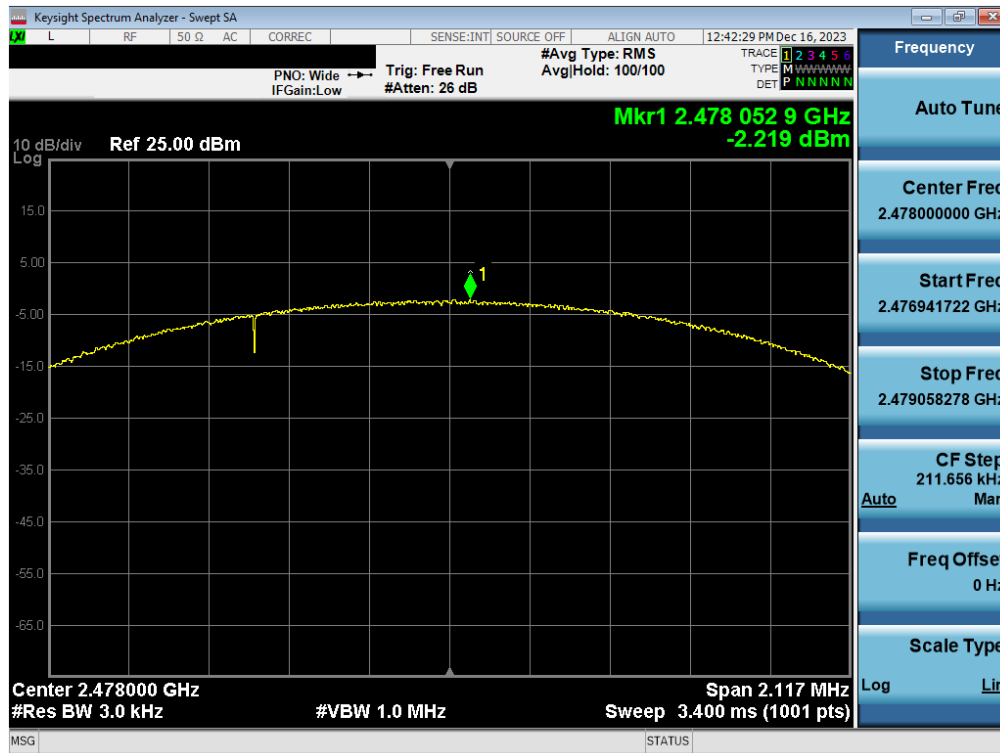
Plot 7-21. Power Spectral Density Plot Antenna WF7b (Bluetooth (LE), 2Mbps, ePA – Ch. 38)
