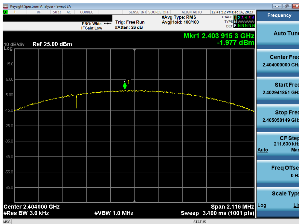
Plot 7-19. Power Spectral Density Plot Antenna WF7b (Bluetooth (LE), 2Mbps, ePA – Ch. 1)
