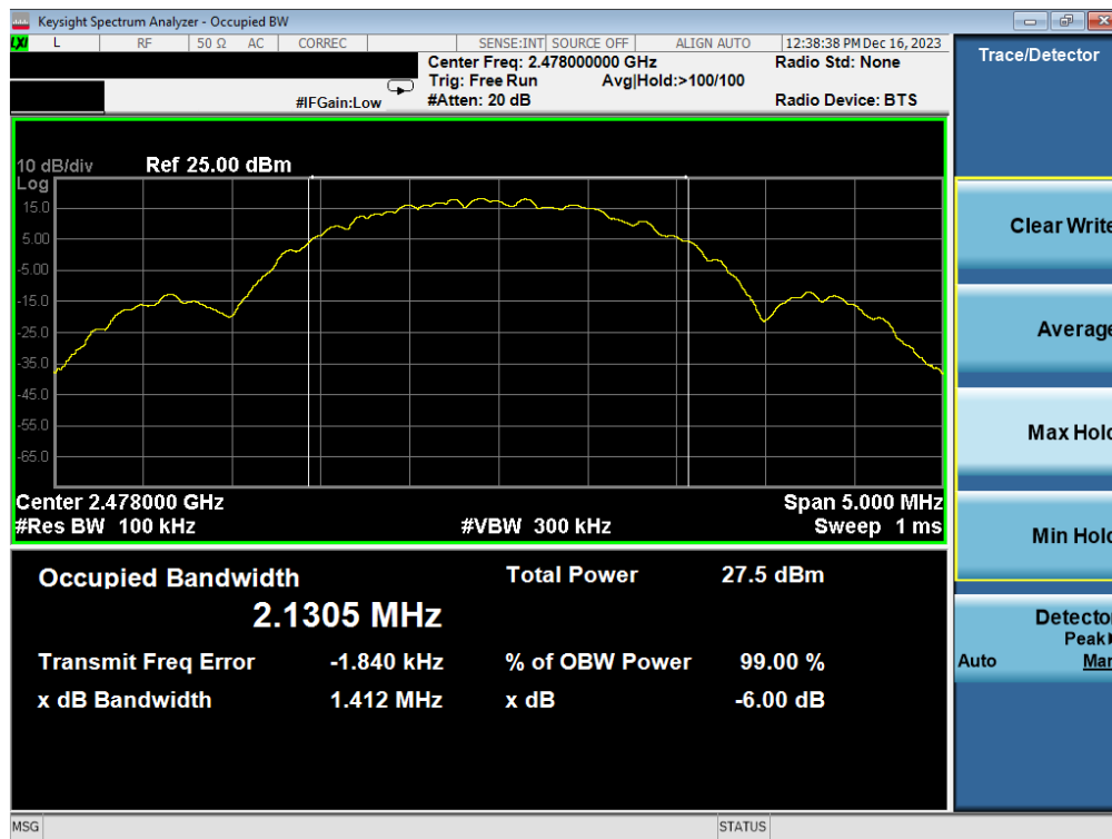
Plot 7-6. 6dB BW & 99% OBW Plot Antenna WF7b (Bluetooth (LE), 2Mbps, ePA – Ch. 38)
