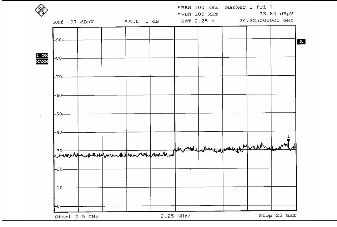
**802.11g OFDM modulation (Both chains on with Antenna 2)**
