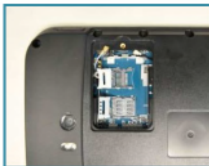
Figure 2-6 Open the lid and insert the mSD card into the slot
