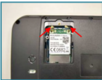
Figure 2-3 Open the aerial terminals on the both sides above.
