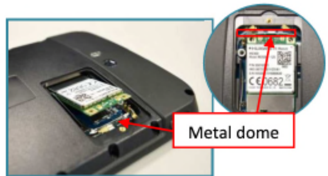
Figure 2-4 Press the metal dome above to flip the module out.
