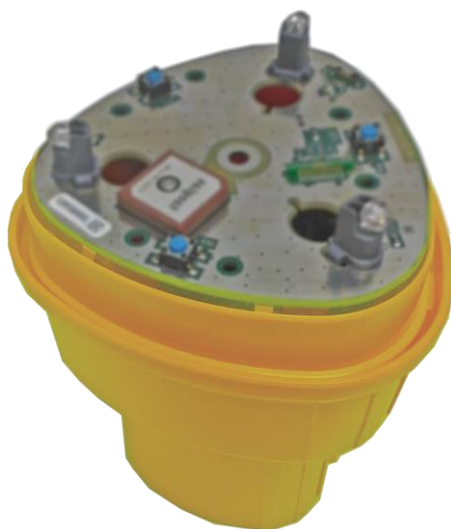
Figure 10 - Kannad Internal photo1
