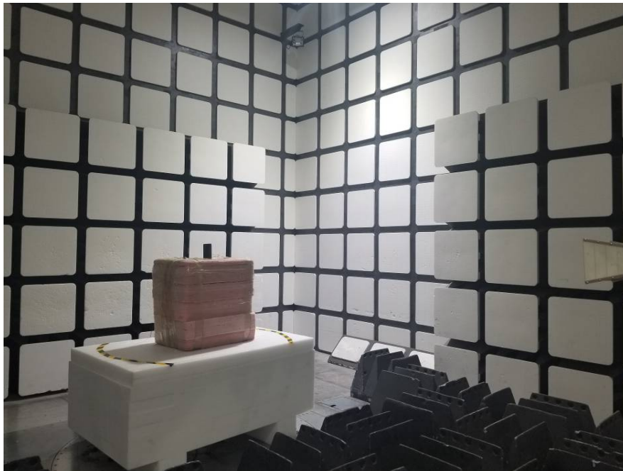
Radiated Emissions View (Above 1 GHz)
