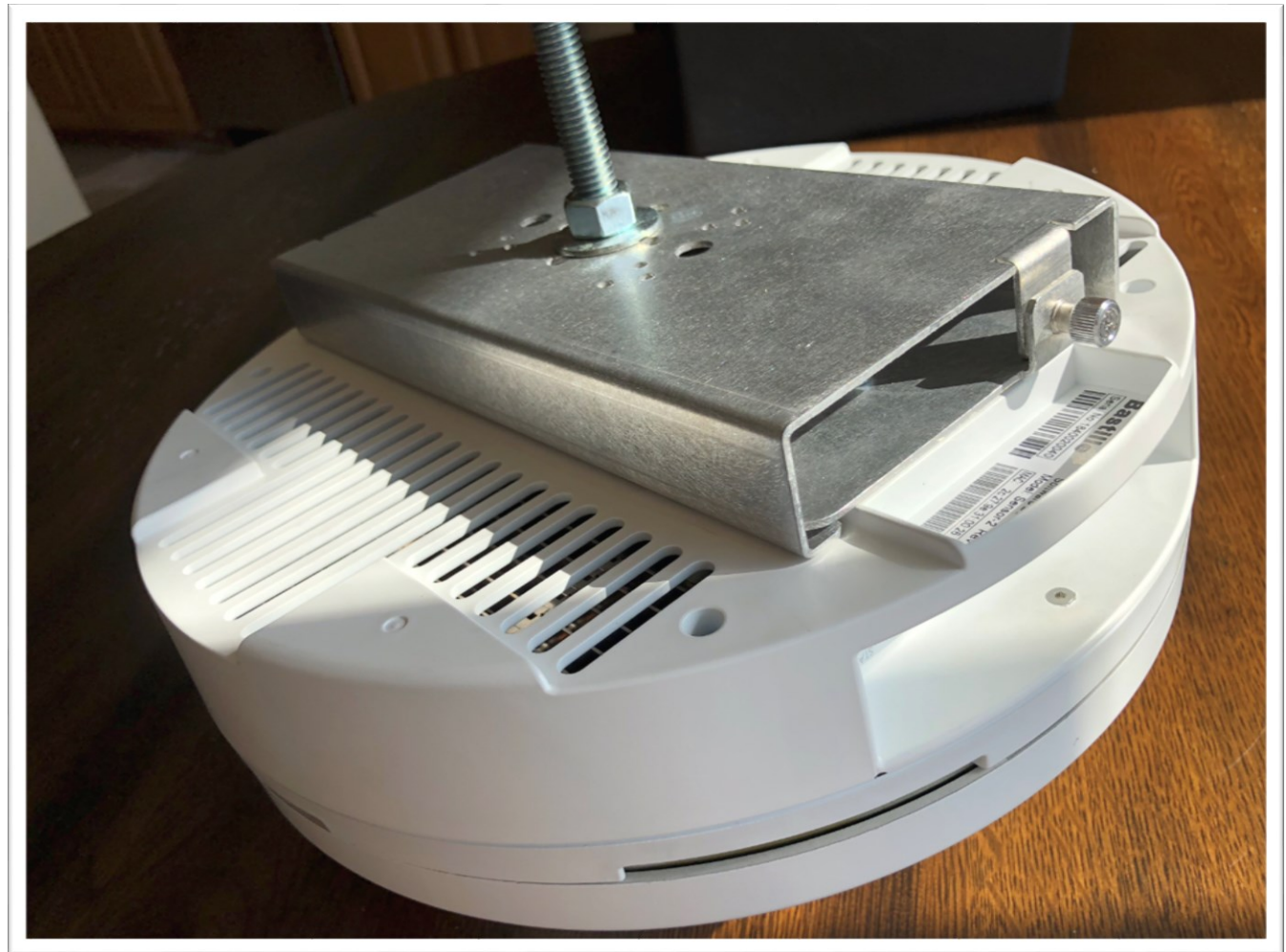
Figure 10. Mounting Plate Fully Inserted to Adapter Plate.
