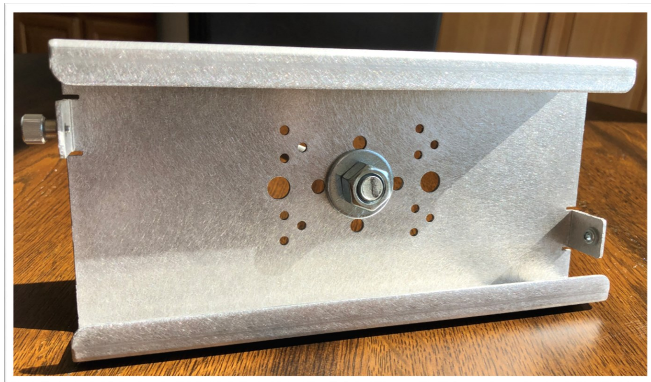
Figure 8. Sensor-02 Adapter Plate Attached to Threaded Rod (bottom view)
