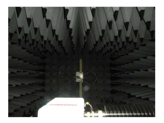
PHOTOGRAPH 3: Test place configuration for testing radiation emission 0.3 – 1.0 GHz
