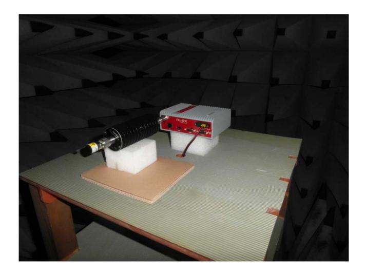
PHOTOGRAPH 2: Test place configuration for testing radiation emission 30 - 300 MHz
