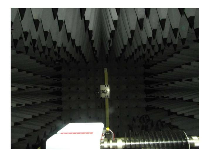
PHOTOGRAPH 4: Test place configuration for testing radiation emission over 1.0 GHz
