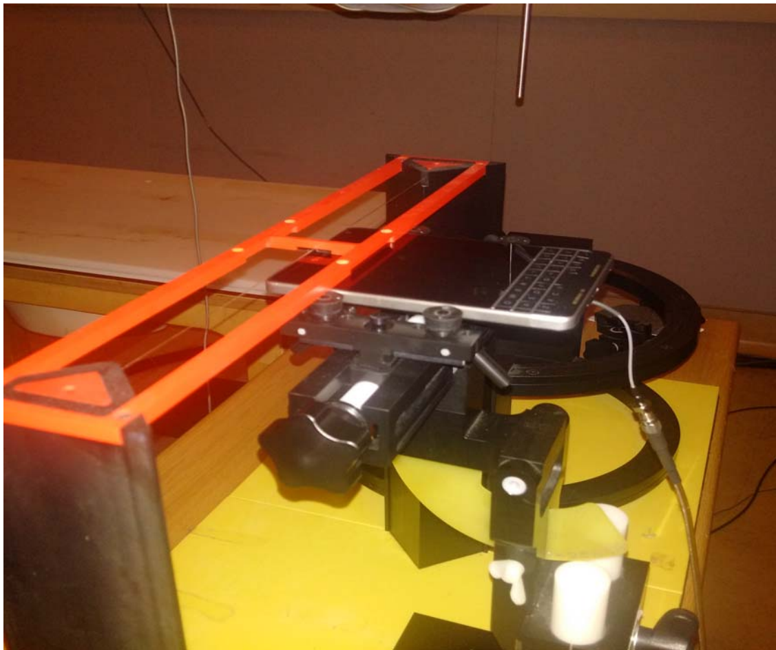
Figure E3: Audio Band Magnetic (ABM) T-Coil measurement setup
