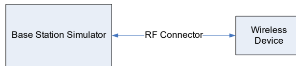
Figure 9-3 Power Measurement Setup
