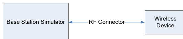
Figure 9-1 Power Measurement Setup
