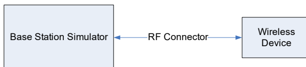
Figure 9-2 Power Measurement Setup
