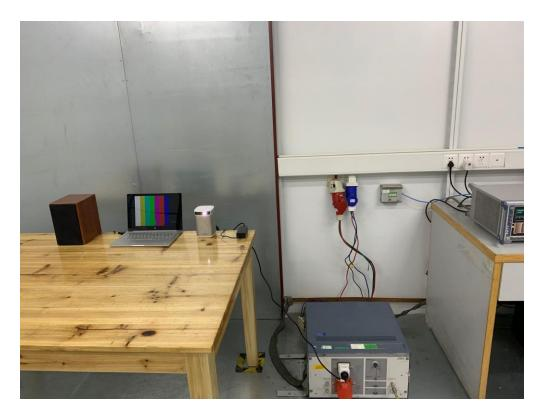
FCC RADIATED EMISSION TEST SETUP BELOW 1GHZ
